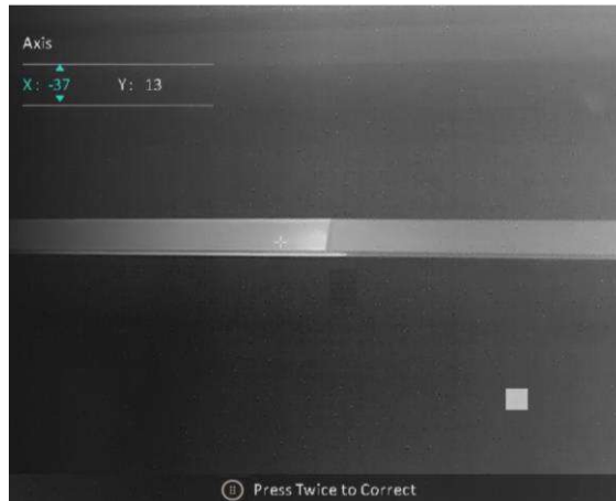
Figure 3-6 Correct Defective Pixel
